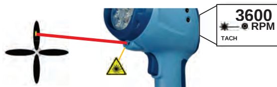
Figure 7 Using the Laser Module
