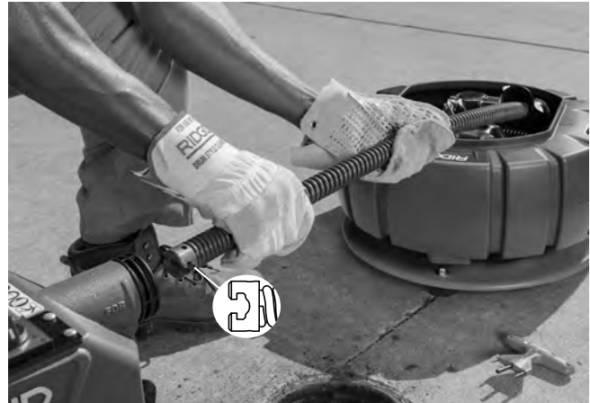
Figure 7 – Inserting Cable Into Front Of Machine
