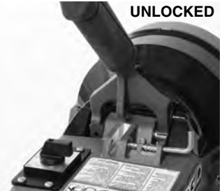
Figure 4 – Releasing the Clutch Handle
