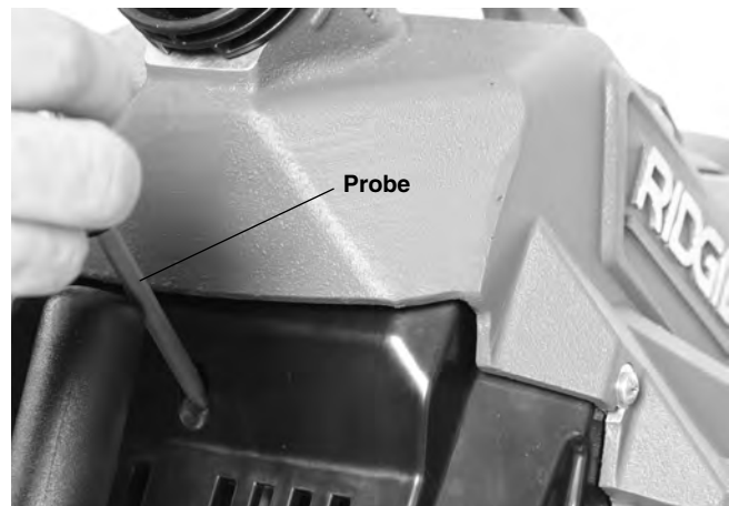
Figure 22 – Motor Reset Button
