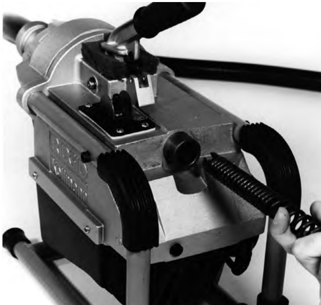
Figure 5 – Inserting Cable Into Front Of Machine
