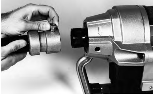
Figure 4 – Rear Guide Hose Attachment
