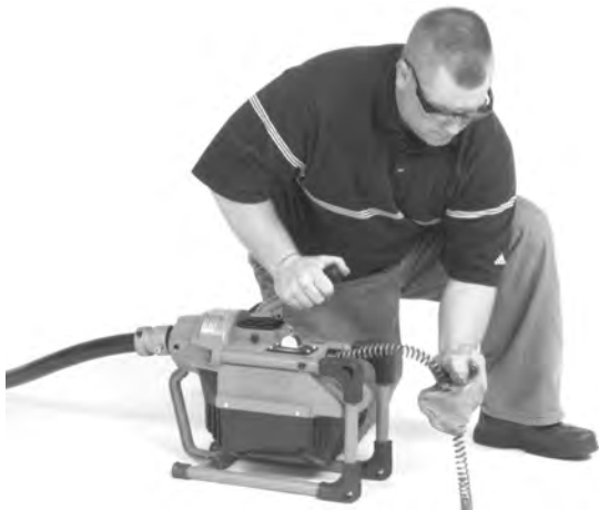
Figure 7 – Proper Operating Position
