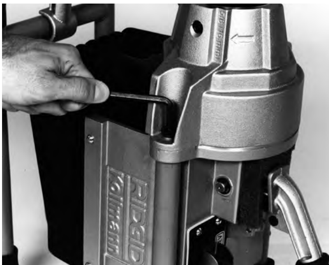
Figure 11 – Remove Socket Head Cap Screws
