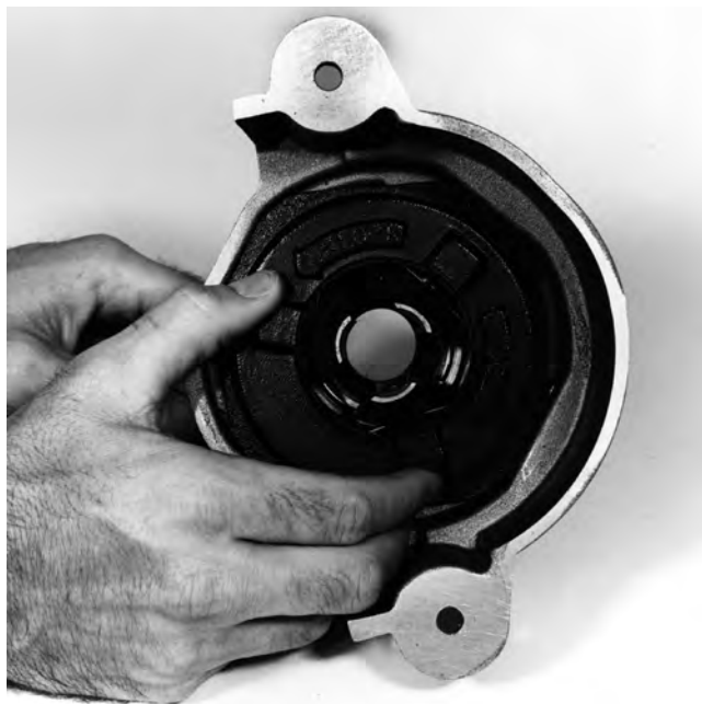
Figure 12 – Remove Jaw Set Cover
