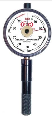
Model 601 Pencil Style Analog Asker C Durometer with 0 to 100 point dial and 1/2" diam. base.
