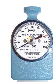
Model 603 Classic Style Analog Asker C Durometer has an easy to read 0 to 100 point dial and 1/2" x 2" base.
