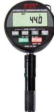
Model 611 Pencil Style Digital Asker C Durometer features easy to read LCD dial and 1/2" diam. base.
