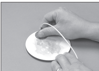
11.19 Polish the connector for four to eight figure eights only.
