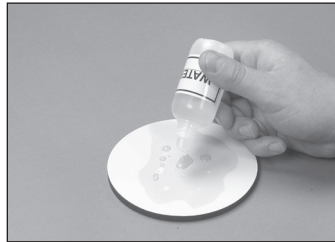
11.14 Final Polish: Clean the lapping film with a lint free cloth and distilled water. Add several drops of distilled water onto the lapping film.
