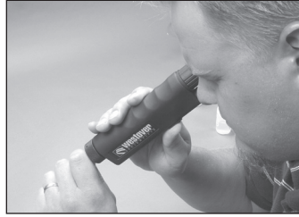
10.11 Inspect the connector endface with the fiber through coaxial and oblique views by changing the view with the thumbswitch on the body of the 3M View Scope.
