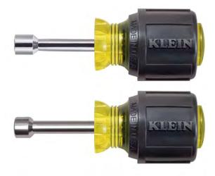
Tool Set includes two nut drivers (Cat. No. 610-1/4 and 610-5/16). Full hollow shank for long bolts or studs. Stubby nut drivers allow for work in close quarters. Color-coded handles for easy identification. Meets or exceeds applicable AMSE / ANSI specifications.
