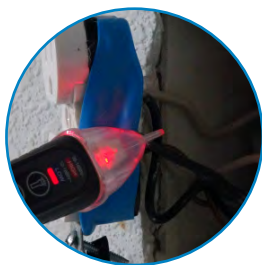
Detects AC voltage on conductors
