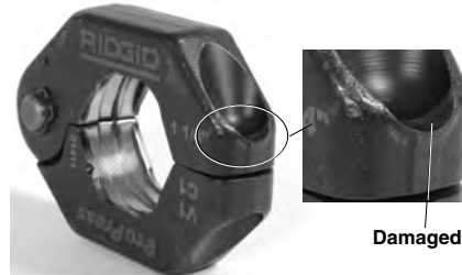
Figure 11 – Damaged Ring Pocket
