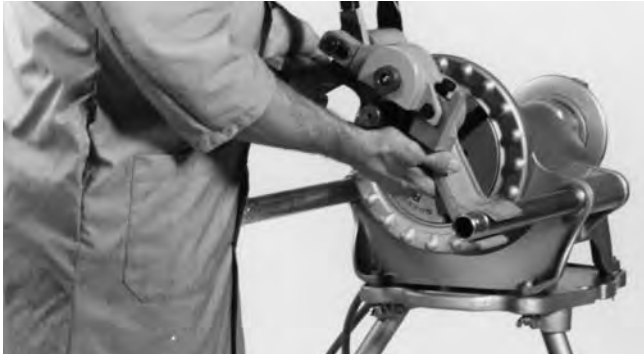
Figure 2 – Mounting on No. 300 Power Drive
