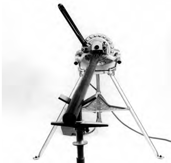
Figure 8A – Operating Machine in REVERSE (REV) Position
