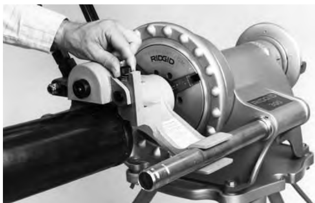
Figure 10 – Loosen Depth Adjustment Screw
