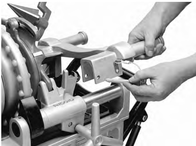
Figure 5 – Attaching Adapter Bracket to 300 Compact Threading Machine
