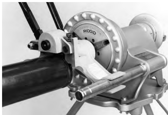
Figure 9 – Feed Handle in UP Position
