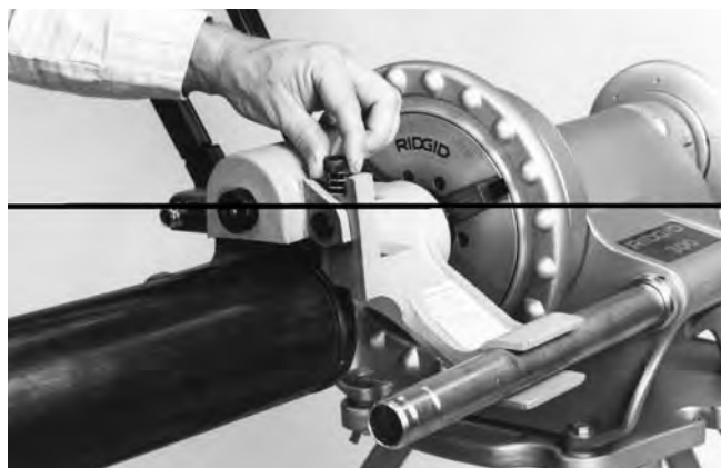
Figure 11 – Tighten Depth Adjustment Screw
