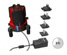
Charge the Li-Ion battery before using it for the first time. While charging, the instrument may heat up. This is normal and should not affect the instrument's lifespan or performance. At the recommended storage temperature of -20°C to +30°C (-4°F to +86°F), batteries containing a 50% to 100% charge can be stored up to 1 year. After this storage period the batteries must be recharged.
