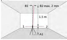
Set up the laser on its tripod o wall mount bracket near point A1 at a minimum distance of 1.5 m from point B1. The horizontal laser is aligned in direction 1. Mark the laser points A1 and B1 with a
