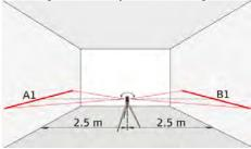
Set the instrument on a tripod half-way between two walls (A+B) that are approx. 5 m apart. Place the lock switch in the "Unlocked" position. Direct the instrument at wall A and switch on the instrument. Activate the horizontal laser line or laser point and mark the position of the line or the point on wall (A1). Rotate the instrument by 180° and mark the horizontal laser line or the laser point in exactly the same way on wall (B1).
