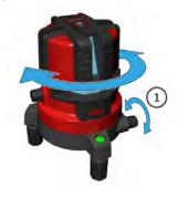
Turn adjustment knob (1) for fine adjustment of vertical laser lines.
