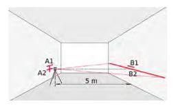
Then place the instrument at the same elevation as close as possible to wall A and again mark the horizontal laser line or the laser point on wall A (A2). Rotate the instrument by 180° again and mark the laser on wall B (B2). Measure the distances of the marked points A1-A2 and B1-B2. Calculate the difference of the two meas-
