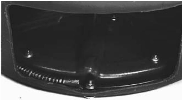
Figure 24 – Anchoring of Pigtail in Drum
