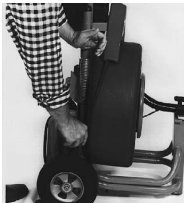
Figure 18 – Release Belt Tension
