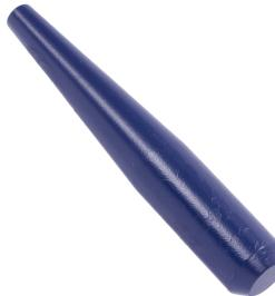
Klein Tools Barrel Drifts are designed for aligning holes in construction. They can also be used for expanding holes in mild steel. The taper is forged, not turned, for greater tensile strength.
