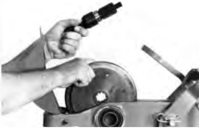
Figure 12 – Remove Cutter Wheel Assembly
