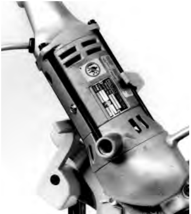
Figure 5 – Position Power Drive Inside Reaction Arm
