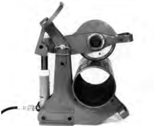
Figure 8 – Positioning Pipe in Cutter
