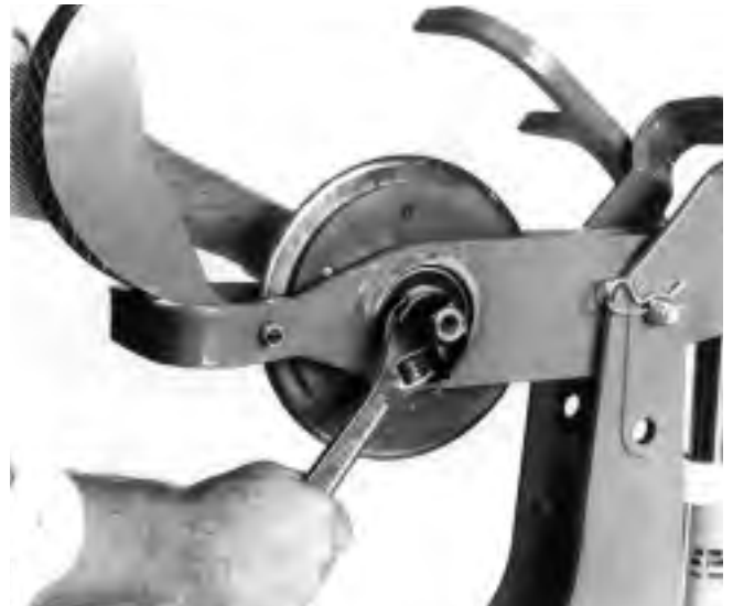
Figure 11 – Remove Locking Nut
