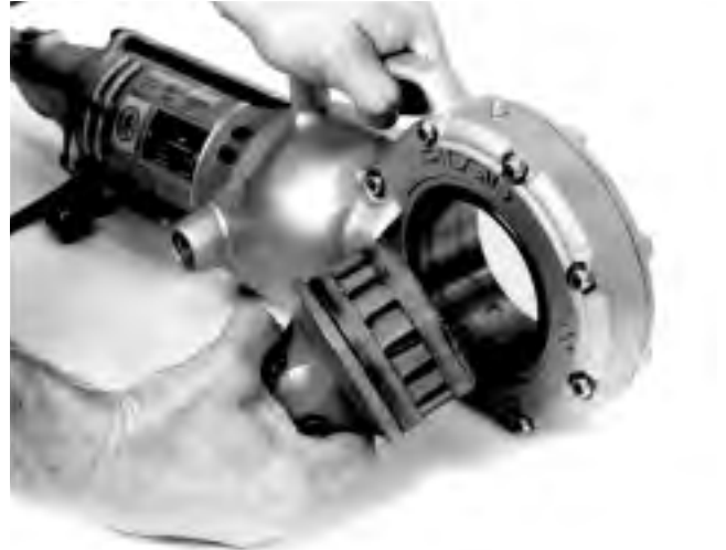
Figure 4 – Installing 774 Drive Adapter
