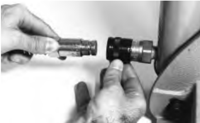
Figure 3 – Connecting Hydraulic Foot Pump to Cutter
