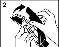
Open the knife to replace cutting blades and reveal the replacement blade compartment.
