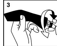
Slide knife halves back together and rotate back end of knife to original position to close and lock.
