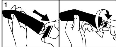
Make sure the blade is retracted before opening the knife. Pull back end of knife and rotate to release and open the two parts of the knife.
