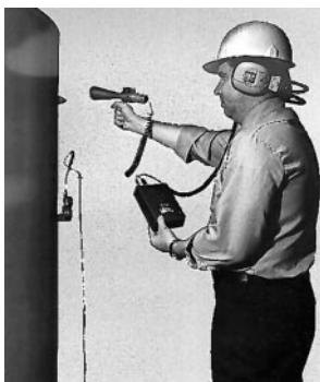
Locating a leak in an air pressure tank
