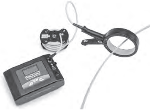
Figure 14 – Inductive Clamp Attached to a Conductor
