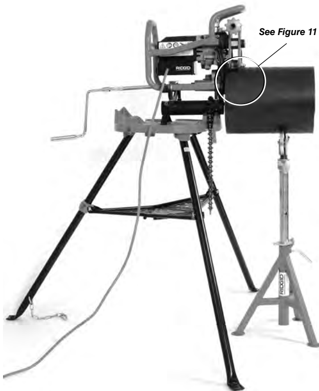
Figure 12 – Fixed Beveller, Short Pipe, One Pipe Stand
