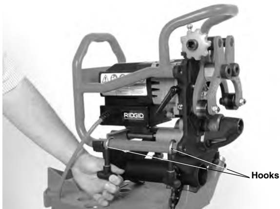
Figure 9 – Securing Beveller to Adapter
