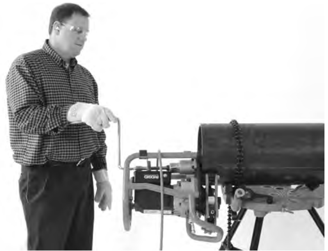
Figure 20B – Bevelling Operation (Fixed Workpiece/Moving Beveller)
