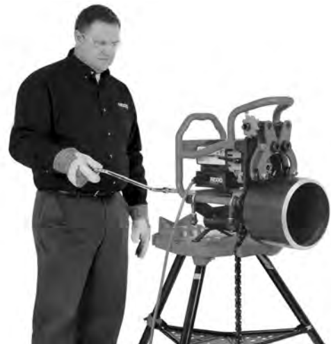
Figure 20C – Bevelling Operation (Fixed Beveller/Rotating Pipe)
