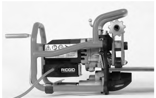
Figure 16B – Installing Beveller on Plate
