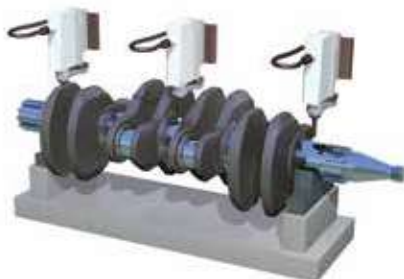
7 Workpiece runout measurement
