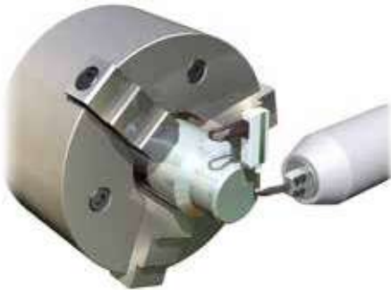
3 Machine device tool length measurement
