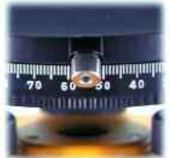
Compensator Lock Protects Instrument During Transport
