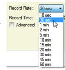
Sample Rate - If you check the Advanced radio button the Advanced options will be shown – see right. This allows the User to choose a sample rate, which is the rate at which the logger takes a sample of whatever it is recording e.g. Temperature. This sample rate is independent of the Record Rate described above. The sample rate is always less than or equal to the record rate. For this example the
