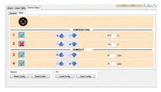
This is the Alarm window from a Temperature/Humidity logger. It has two alarms per channel. The alarms are numbered 1 and 2 for Temperature and 3 and 4 for Humidity.
