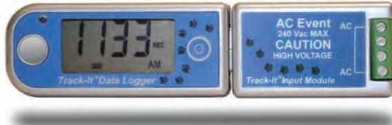
The Track-It™ AC Event Logger can also be used to record ambient temperature along with on/off cycles. This can help diagnose heat vs. cycle time issues. Information displayed on the LCD is also user programmable and can be sequenced by pressing the logger button. The multicolor LED indicator notifies the user of temperature alarms or general activity.
