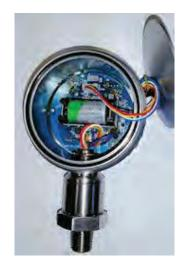
The unit operates off a 1/2 AA 3.6V Lithium battery. The battery is accessed by removing the rear bezel ring and cover. Gently extract the battery and replace as needed. NOTE POLARITY WHEN REPLACING - the unit will not operate if the battery is reversed. Ensure the O-ring is in place before replacing the cover and bezel. Do not stress any of the internal wiring.
