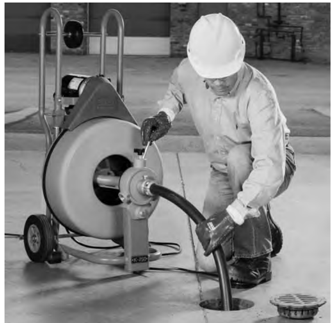
Figure 15 – Using Machine with Guide Hose
