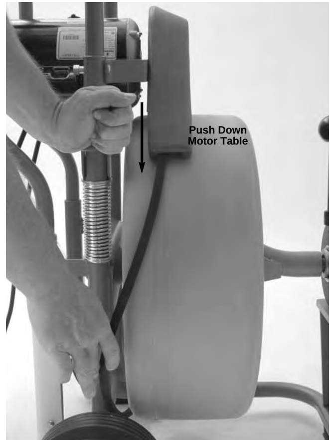
Figure 17 – Releasing Belt Tension
