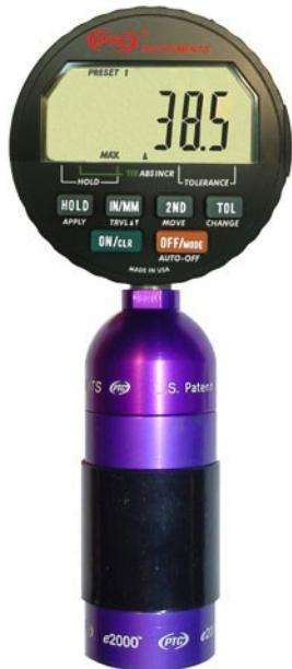
ASTM type B durometer gauges measure the hardness of skate wheels, printing platen, rubber, thermoplastic, and elastomers.
