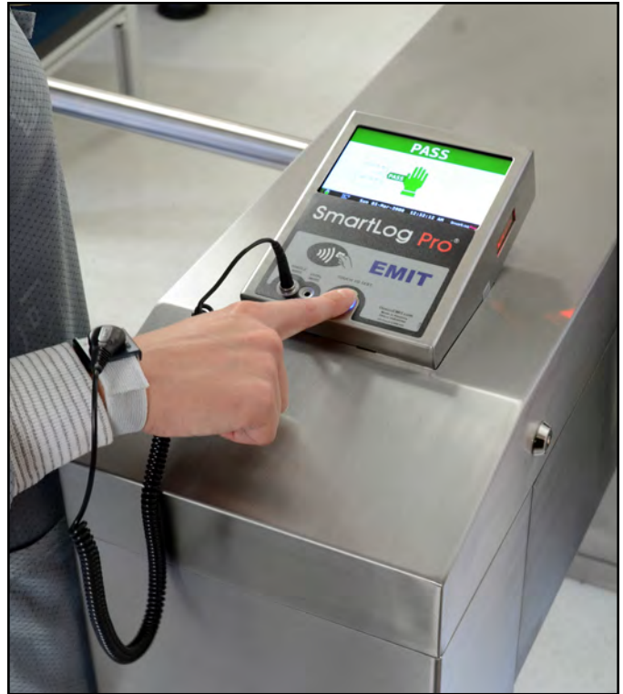
Figure 7. Performing a single-wire wrist strap test
