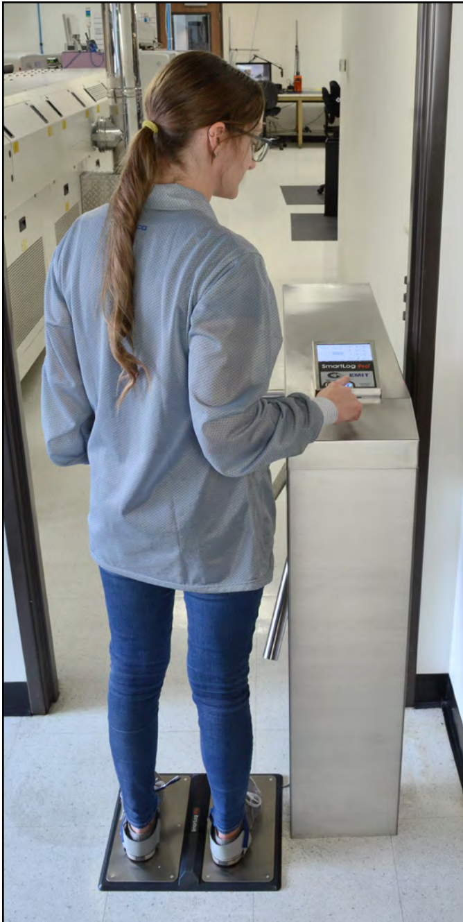
Figure 6. Performing a footwear test
