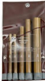
Klein Tools' Brass Punches are designed for applications requiring a softer punch. Or more specifically, any situation where using a hardened punch may cause damage. The brass composition is specially selected for punch use.
