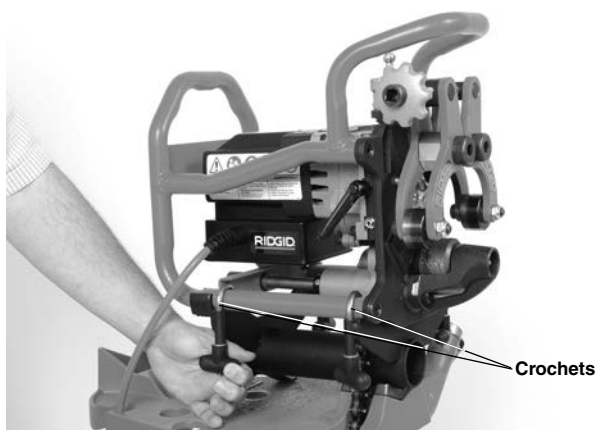
Figure 9 – Securing Beveler to Adapter
