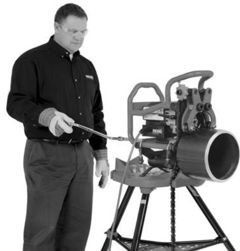
Figure 20C – Bevelling Operation (Fixed Beveller/Rotating Pipe)
