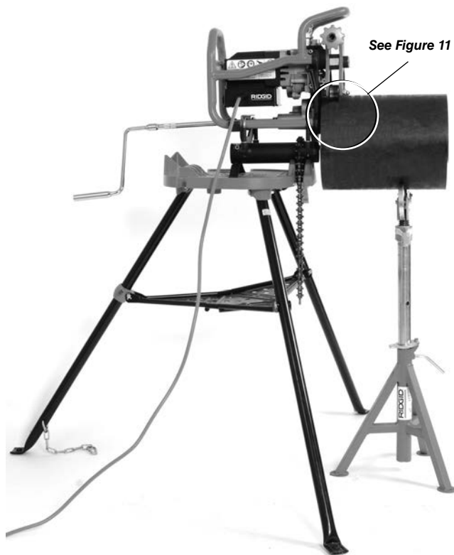
Figure 12 – Fixed Beveller, Short Pipe, One Pipe Stand
