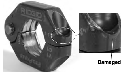
Figure 11 – Damaged Ring Pocket
