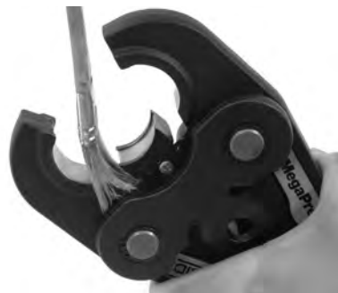
Figure 13 – Cleaning Segment Area of MegaPress Jaw
