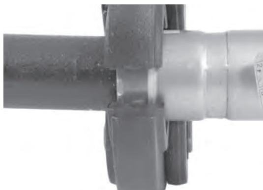
Figure 9 – MegaPress Jaw Set Square To Fitting and Tubing
