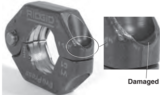
Figure 11 – Damaged Ring Pocket
