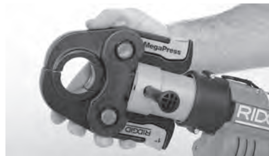
Figure 4 – Sliding The Attachment Out of the Tool
