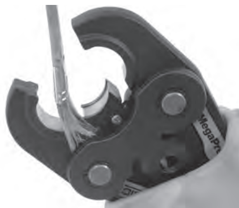
Figure 13 – Cleaning Segment Area of MegaPress Jaw
