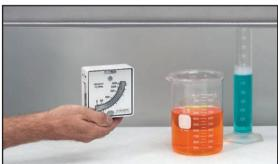
Use a Vaneometer<sup>TM</sup> Swing Vane Anemometer to measure velocity of air flow into laboratory fume hoods and at paint spray booths to determine when to change filters. Or wherever needed to meet OSHA standards of ventilation for smoke, dust or fume removal.
