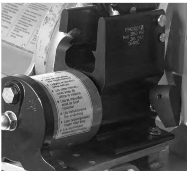
Figure 9 – Close-Up of Release Lever on 918 Pump
