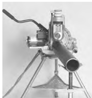
Figure 12 – Offset Pipe on 918 in FORWARD Position
