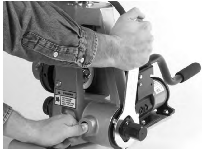
Figure 19 – Engaging Spindle Lock and Removing Drive Shaft Retaining Nut
