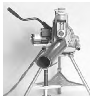
Figure 13 – Offset Pipe on 918 in REVERSE Position
