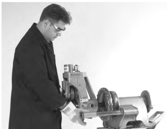
Figure 2 – Installing on 300 Power Drive
