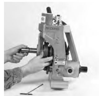
Figure 18 – Removing Retaining Shaft and Groove Roll
