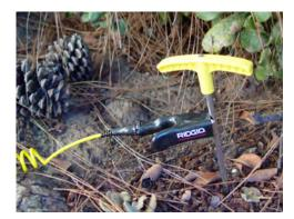
With the transmitter's lead clips attached to the target line and the grounding stake, a circuit is created for the signal to travel. The circuit allows current to flow, energizing the target line.
