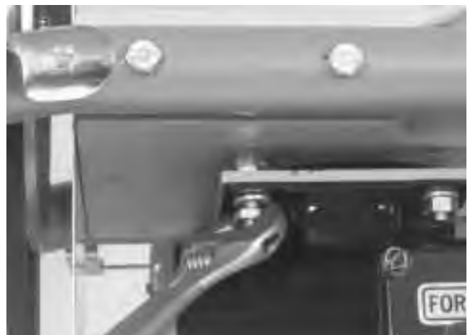
Figure 14 – Removing Clutch End Play
