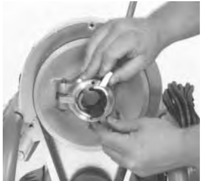
Figure 13 – Replacing Clutch Jaws
