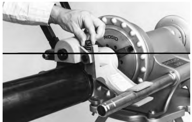
Figure 11 – Tighten Depth Adjustment Screw
