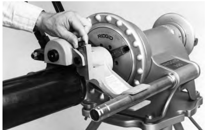
Figure 10 – Loosen Depth Adjustment Screw
