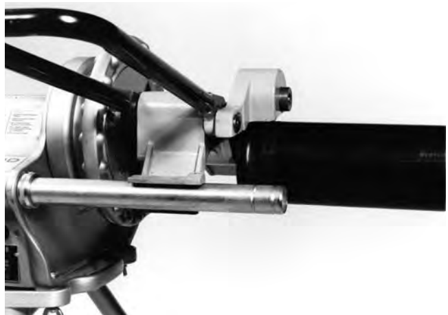
Figure 6 - Square Pipe & Pipe Support
