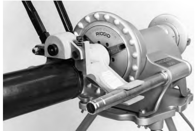
Figure 9 – Feed Handle in UP Position
