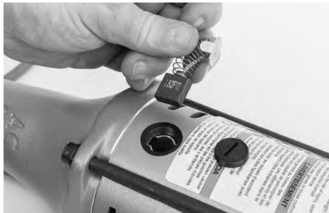
Figure 13 – Installation des balais
