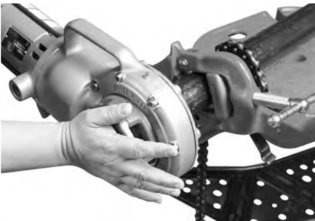
Figure 8 – Starting the Thread
