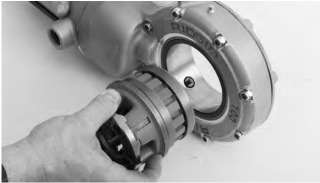
Figure 4 – Installing Die Heads into 700 Power Drive
