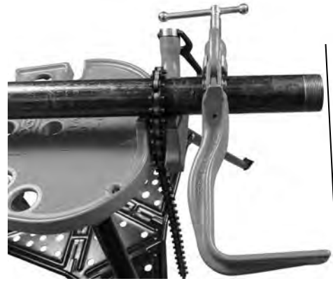
Figure 5 – Support Arm Aligned with End of Pipe
