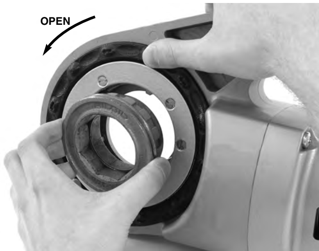
Figure 8 – Installing Adapter Into 690-I
