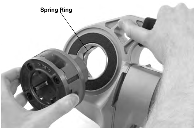
Figure 9 – Installing Die Heads into 600-I Power Drive
