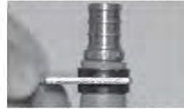
Figure 1 – Hold Gauge Perpendicular To Tube and Slide Over Ring
