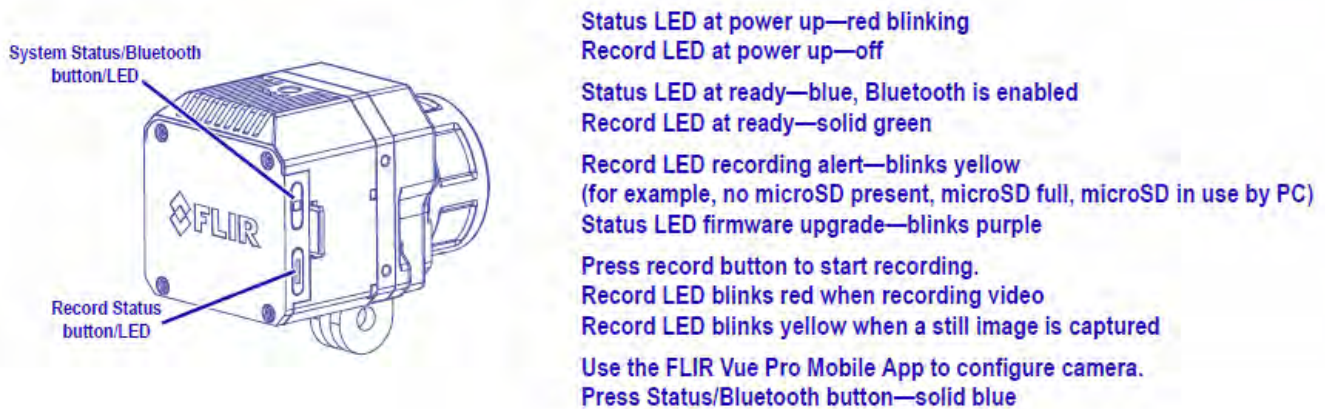
Figure 9. Camera Status and Record LED Description
