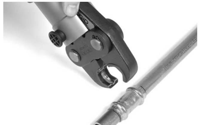
Figure 6 – Opening The Scissor-Style Jaw Set
