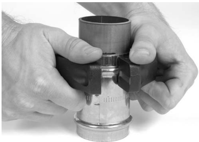
Figure 8 – Installing Press Ring Onto Fitting
