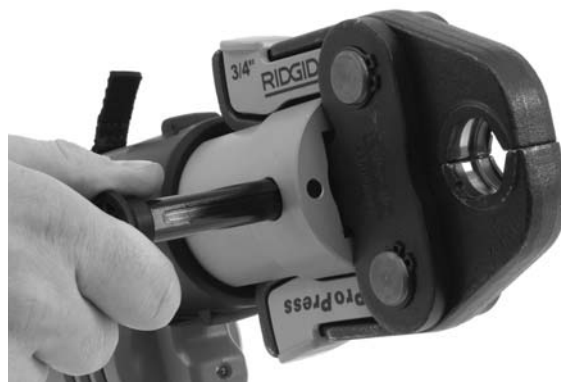
Figure 4 – Fully Open Attachment Mounting Pin
