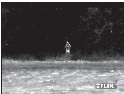
Thermal cameras can complement CCD cameras during the day in situations where contrast is low.
