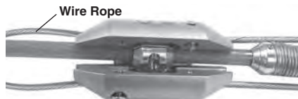
Figure 6 – Locate Pushrod Bulb In Shell
