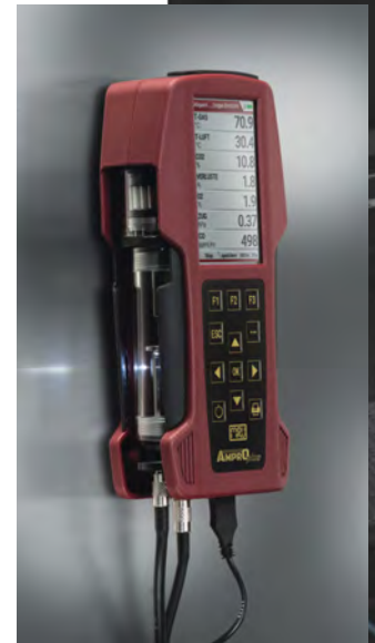
Rear magnets for hand free operation
