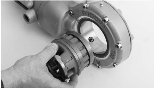
Figure 4 – Installing Die Heads into 700 Power Drive
