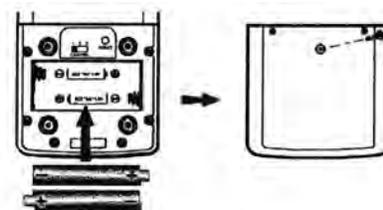
4. Replace the battery compartment door and secure its screws.
