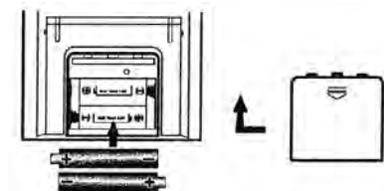
Replace the batteries when the low-battery indicator of the indoor temperature lights up. (Repeat the steps described in section, "Before Beginning".)
