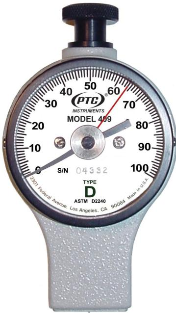
**ASTM Type D Durometers are for determining indentation hardness of Pipeline Coating, Hard Rubber, Acrylic, Delrin, Kevlar, PVC, Nylon, Lexan and Epoxy.**
