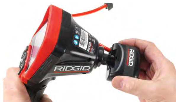
Figure 10 – Connecting the micro CA-300 Camera Monitor
