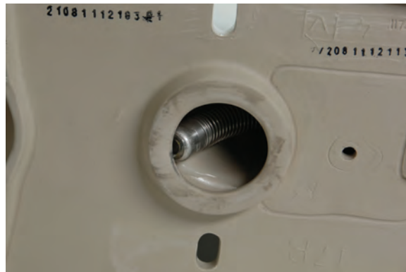
Figure 17 – Camera Head Blocked in Turn
