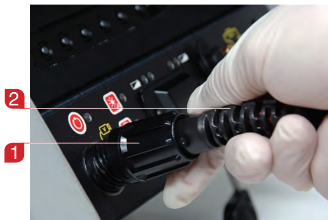
Figure 13 – Connecting to a SeeSnake CCU
