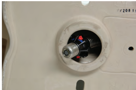
Figure 18 – Camera Head with Ball Guide in Turn
