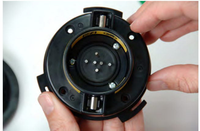
Figure 7 – Broken Contact Pin
