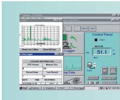
**Leq and SEL measurements with built-in datalogger and PC interface. Datalogs up to 32,000 readings using included software and USB cable.**
