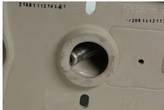
Figure 17 – Camera Head Blocked in Turn
