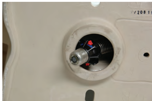
Figure 18 – Camera Head with Ball Guide in Turn
