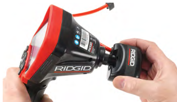
Figure 10 – Connecting the micro CA-300 Camera Monitor
