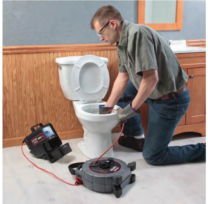
Figure 14 – Performing an Inspection
