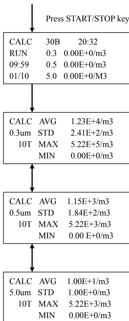
Displayed particle size can be changed by using the ▲▼ key. When “STR” is set to “Y”, the data will be stored in the instrument.
